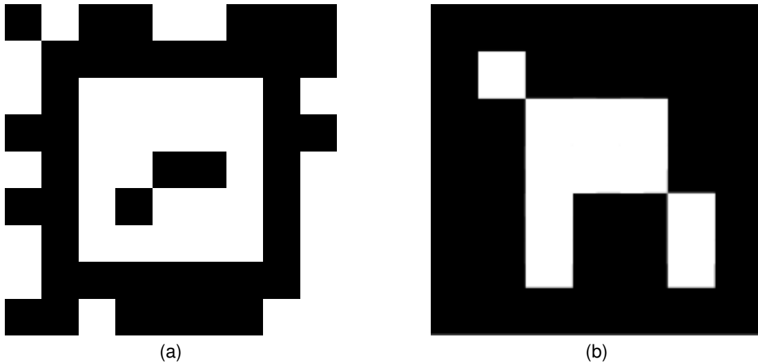
Fig. 1. The fiducial markers used in this experiment (a) AprilTag (ID: 250). (b) ArUco (ID: 250).
